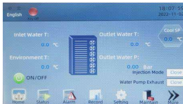
Figure 5-7: Control system homepage interface
